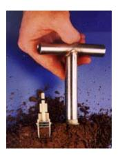
At Left, an attachable, reusable En Core® T-handle is used to push sampler into the soil.
