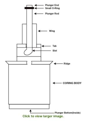
2. Depress locking lever on En Core T-Handle. Place coring body, plunger end first, into open end of T-Handle, *aligning the (2) slots on the coring body with the (2) locking pins in the T-Handle*. Twist coring body clockwise to lock pins in slots. Check to ensure Sampler is locked in place. Sampler is ready for use.
